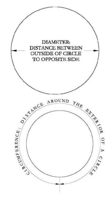
Now that we've re-incarnated your beginnings as a teenager, why are both the diameter and circumference useful to know? Easy, you can measure the diameter of a circle (or in our case piling) when you can get to it. (like when its laying on the ground prior to construction) But if the piling is already installed, and the top of it is 20 ft in the air and the bottom is under 20 ft of water, you can measure the circumference to determine the diameter.
