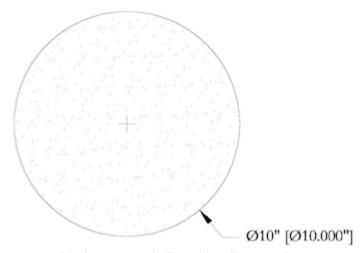
This shows a wood piling with a diameter of 10"
